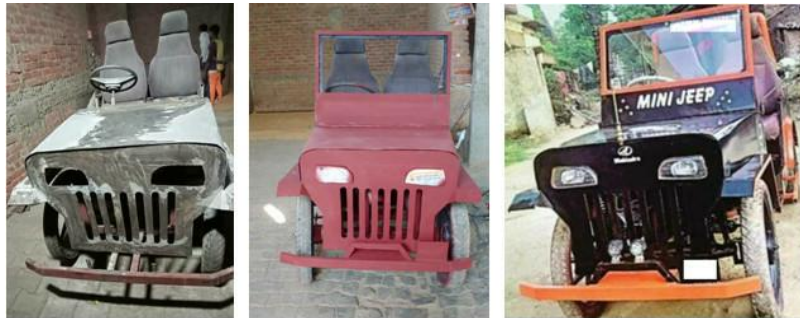
Figure 4: Mini Jeep Fabricated by Students from Motor Cycle Engine
