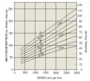
Fig-7 Air Consumption versus Speed
