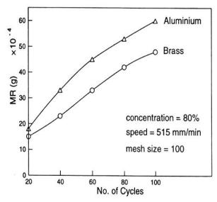
Fig. 3 : Effect of number of cycles on material removal.
