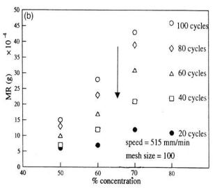
Fig. 4 : Effect of percentage abrasive concentration on material removal at different number of cycles for (a) brass and (b) aluminum as workpiece material.
