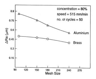
Fig. 8 : Effect of abrasive mesh size on Ra value.
