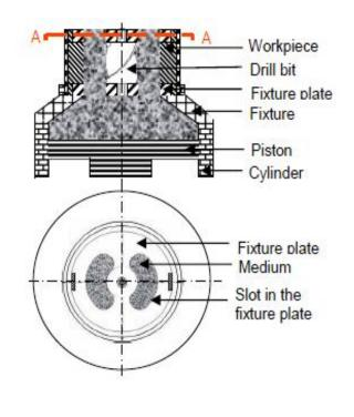
**Fig. 9 :** Sectional front view of tooling in the finishing region in DBG-AFF process and top view of medium splitting through twin slotted fixture plate
