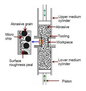
Fig. 1: Abrasive Flow Machining
