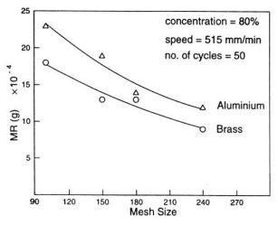
Fig. 5: Effect of abrasive mesh size on material removal.
