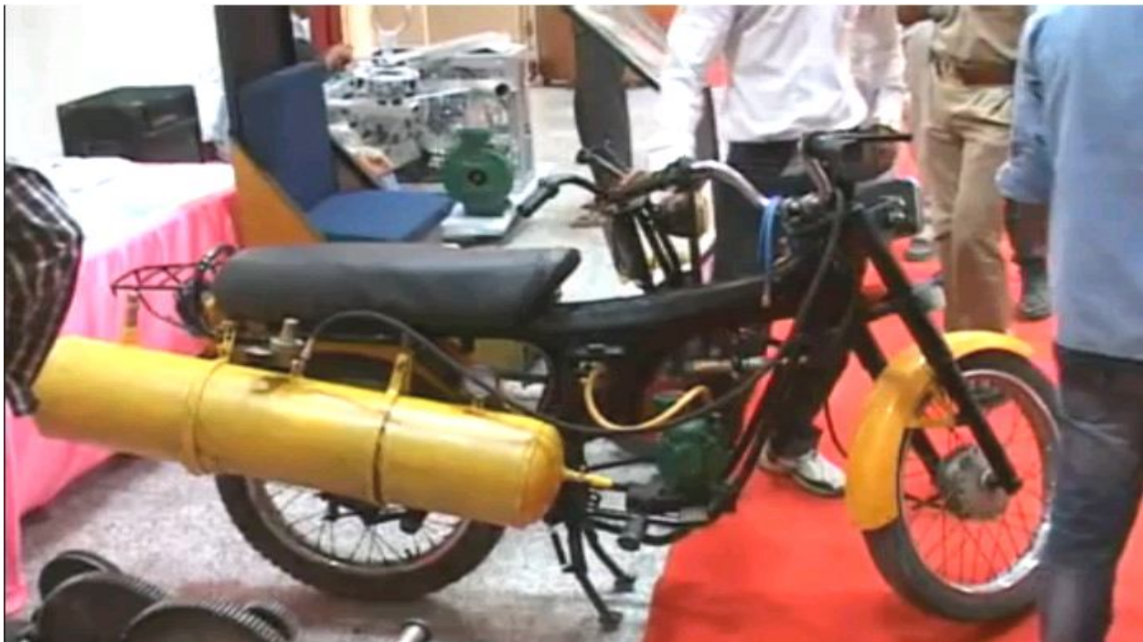
Fig 6: Air-O-Bike- with Storage Cylinder
