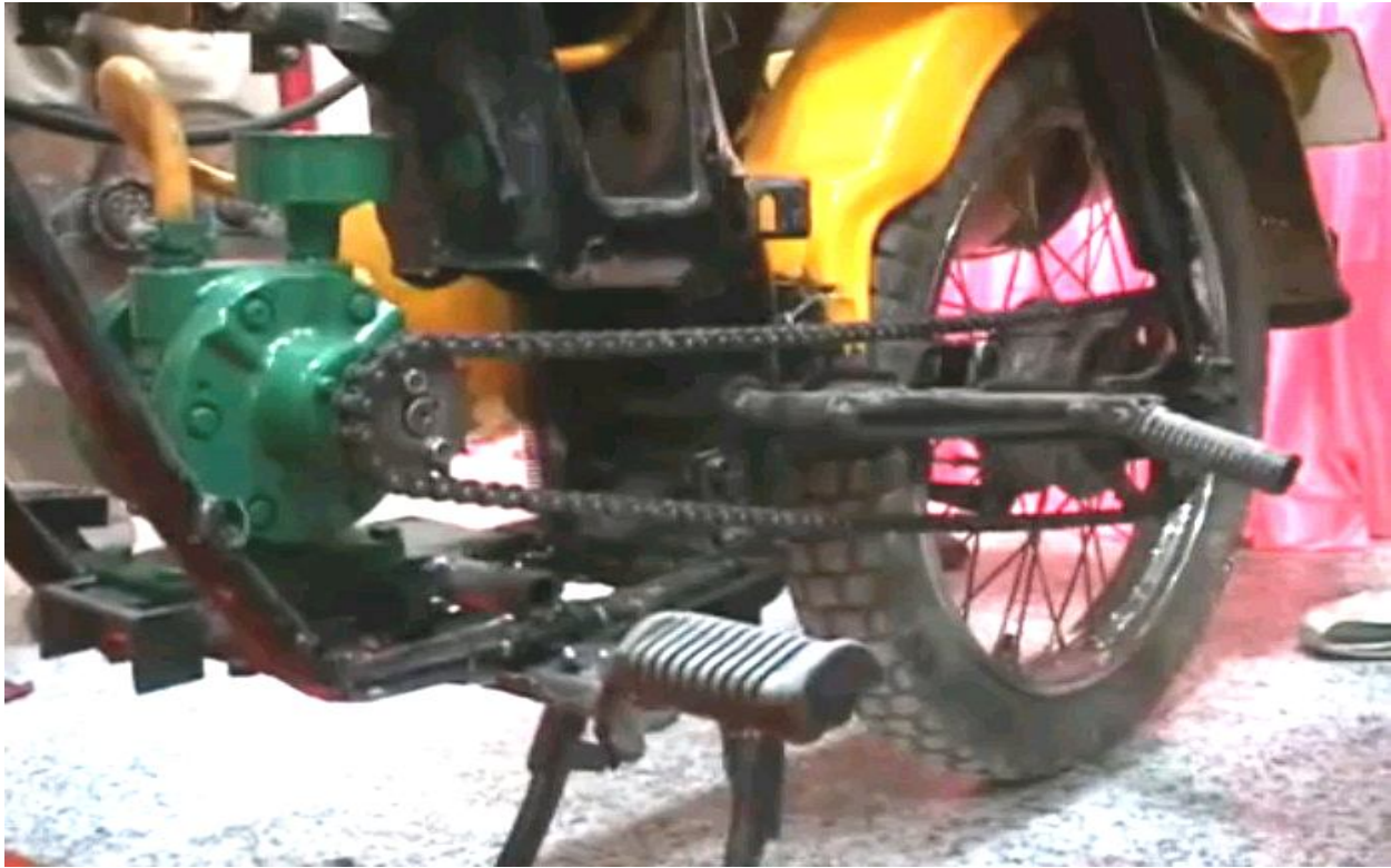
Fig 5: Air -O-Bike- with Air Engine Turbine
