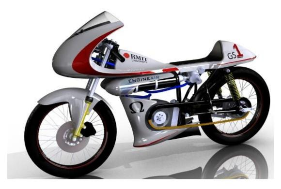
Most motorcycles in the world today use engines that burn gasoline, contributing to greenhouse gasses and adding air pollution to the surrounding area. Now two scientists in India have conceptually designed a new, cleaner motorcycle engine that uses compressed air to turn a small air turbine, generating enough power to run a motorcycle for up to 40 minutes.
