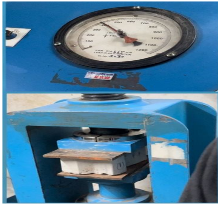
Figure 3: Compressive Test of Paver Block (ZigZag)
