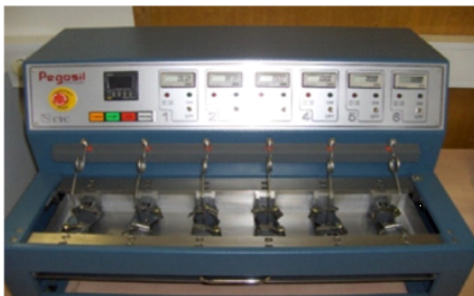
Figure 16: Water absorption testing machine
