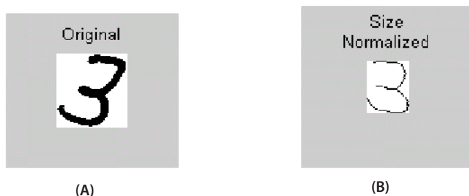
Fig 1.4 :Results after slant correction, thinning and size normalization.
