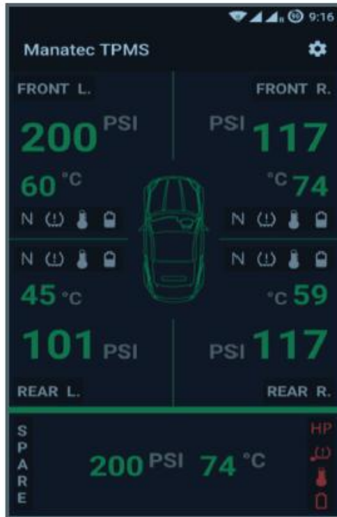
Fig.1.1. Tyre Pressure Monitoring System (TPMS) using Android app
